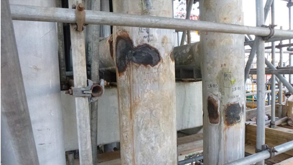
*Corrosion under insulation (CUI) is one of the most insidious problems for offshore assets and one of the most difficult to address (photos courtesy of ClockSpring|NRI)*
