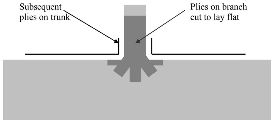
Figure 33. Schematic of repair of tee
