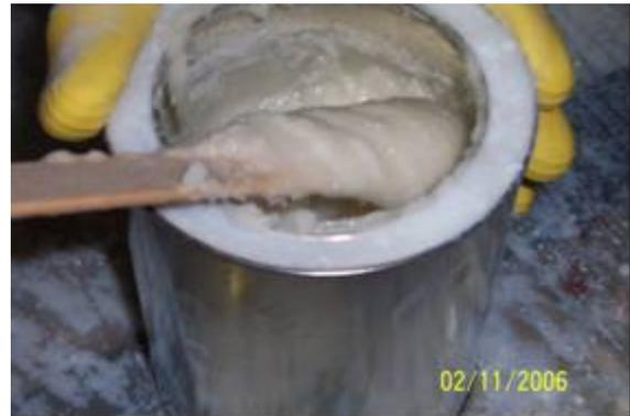
Figure 12. Resin thickened for use as filler
