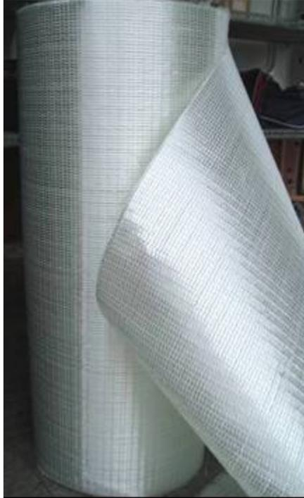
Figure 5. Glass fibre fabric. Note, the fabric is not woven, and so the fibres are not crimped, but lay in flat sheets, to maximise strength and durability
