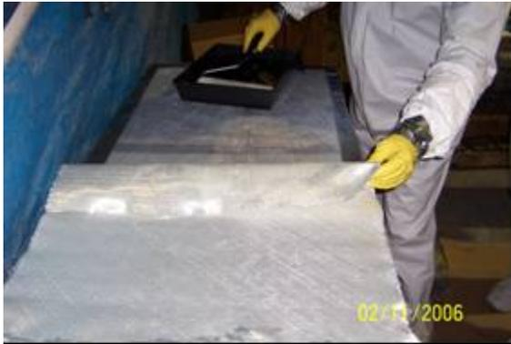
Figure 6. Glass fabric place onto layer of resin (on protected table)
