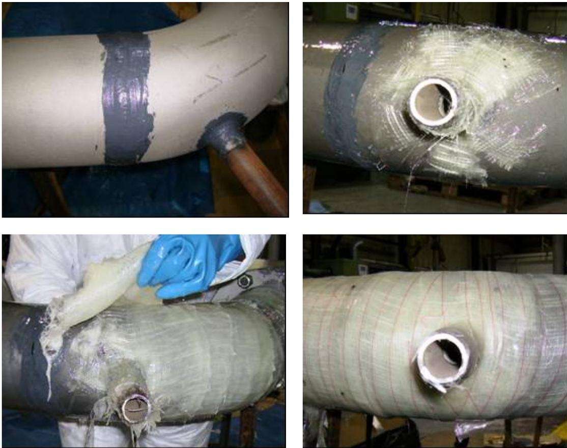
Figure 34. Repair of small bore take off, showing fairing and over-wrap
