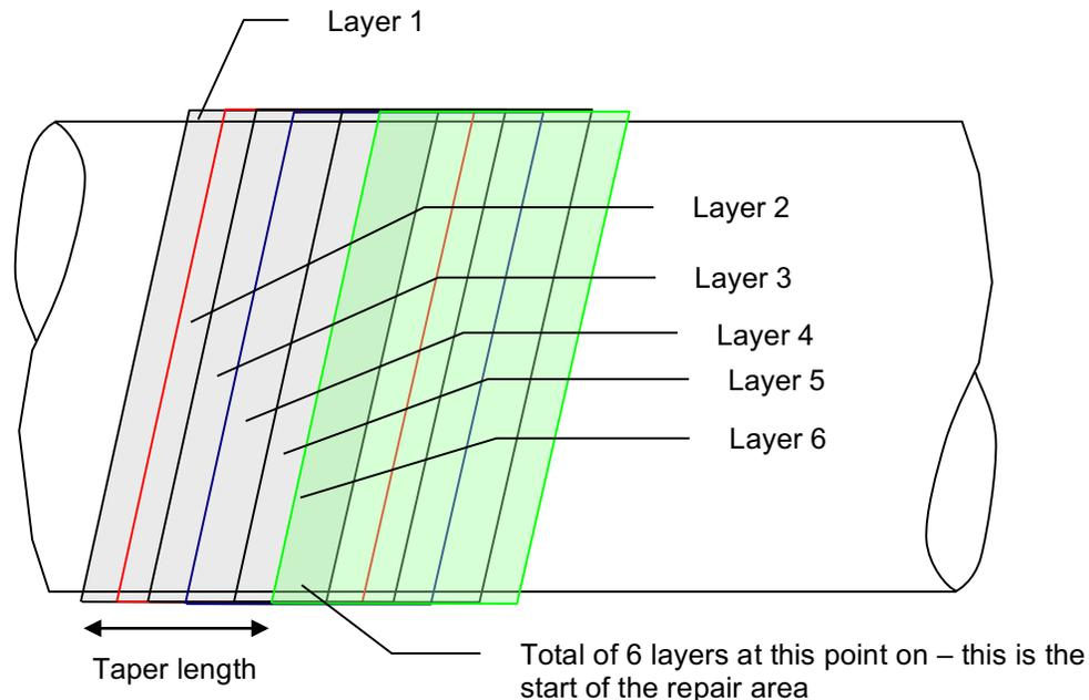
Figure 29. Spiral wrap geometry. Each layer moves on by  $1/6^{\text{th}}$  of the fabric width. Repair starts  $5/6^{\text{th}}$  back from damaged area.
