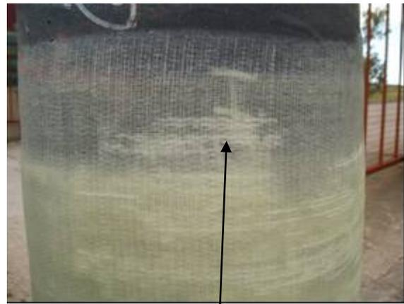
Figure 28. Surface irregularity caused poor wet out and scraping of surface whilst resins till wet
