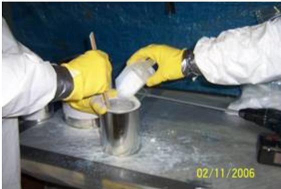
Figure 11. Adding cabosil to resin. Hardener tin was half filled with mixed resin
