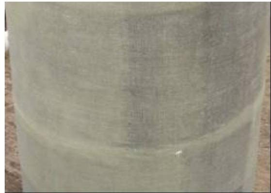
Figure 24. Repair after peel ply has been removed. Overlaps can be seen.
