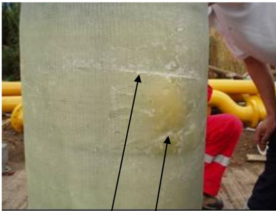
Figure 27. Poor application of peel ply leading to resin uneven surface. Draining resin has created a 'bulge' when trapped in loose peel ply.
