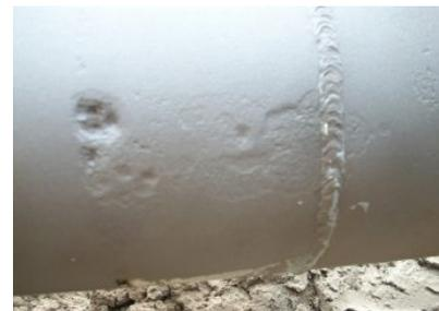
The sand-blasted pipe surface shows corrosion defects.
