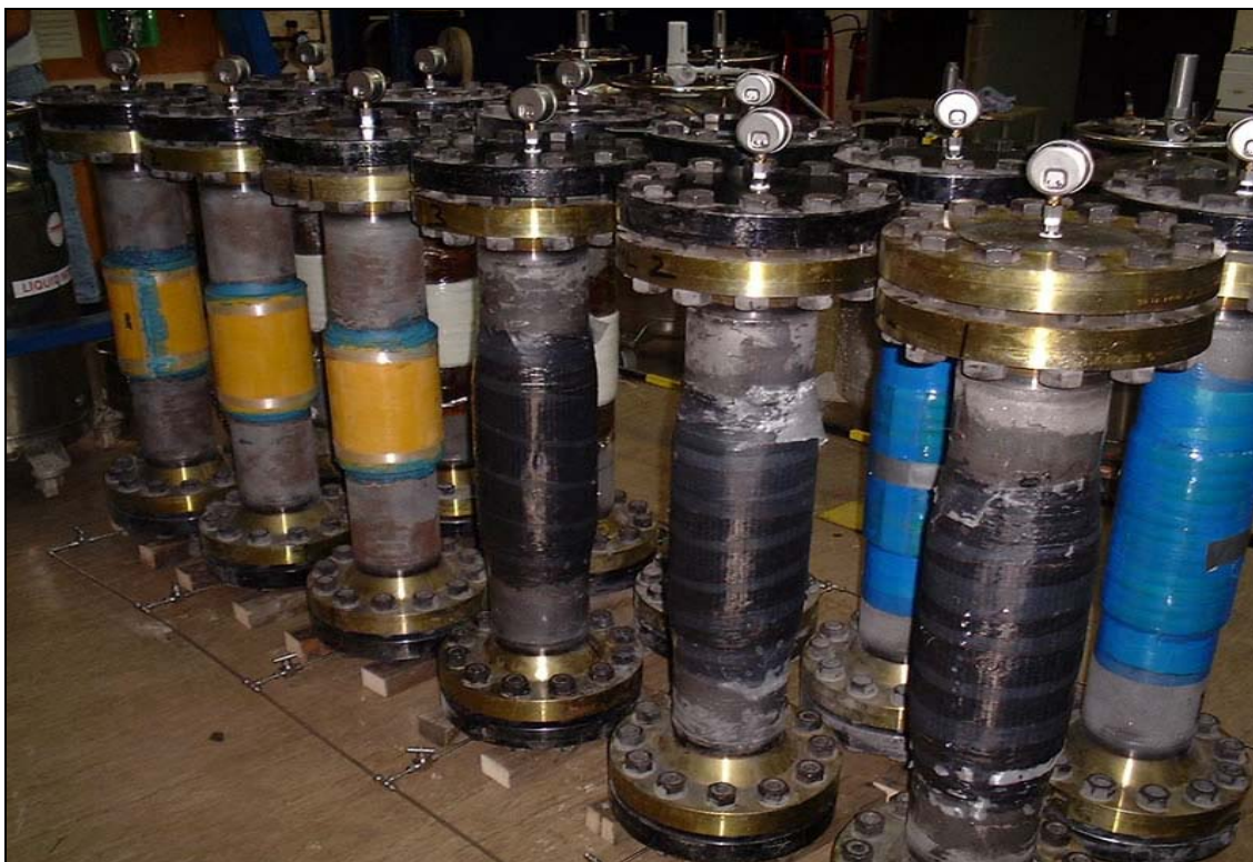
Figure 3: Test spool arrangement
